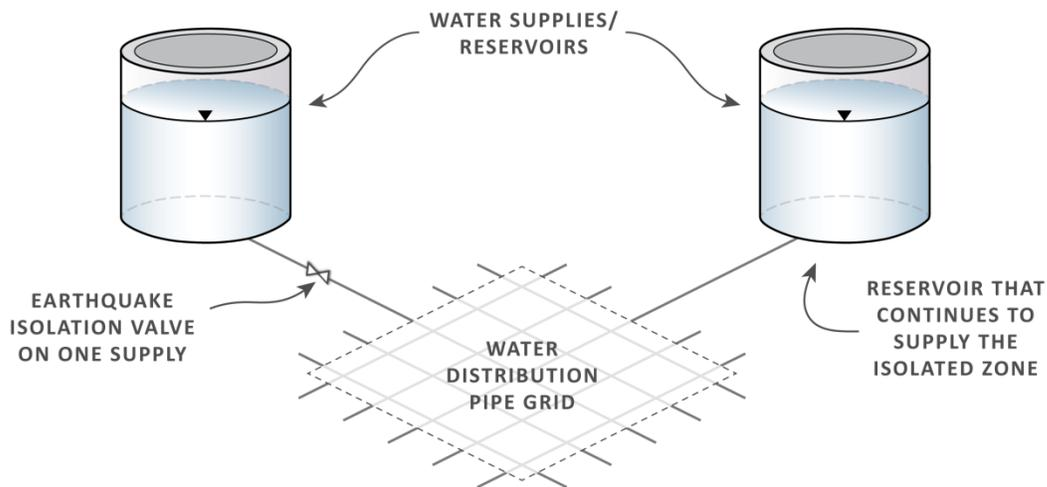
**Figure 4. Typical water distribution system with two supplies/reservoirs, with one earthquake valve**
