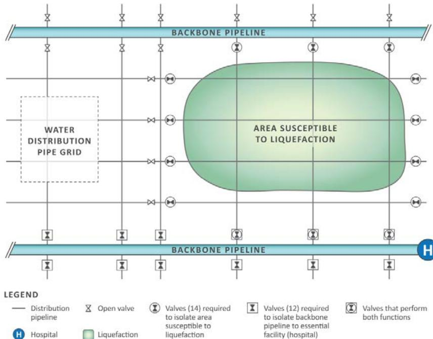
**Figure 5. Valves along backbone pipeline in a typical distribution area**
