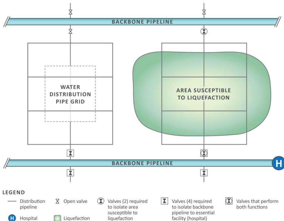
**Figure 6. Arrangement in Japanese distribution system to minimize the number of isolation valves**
