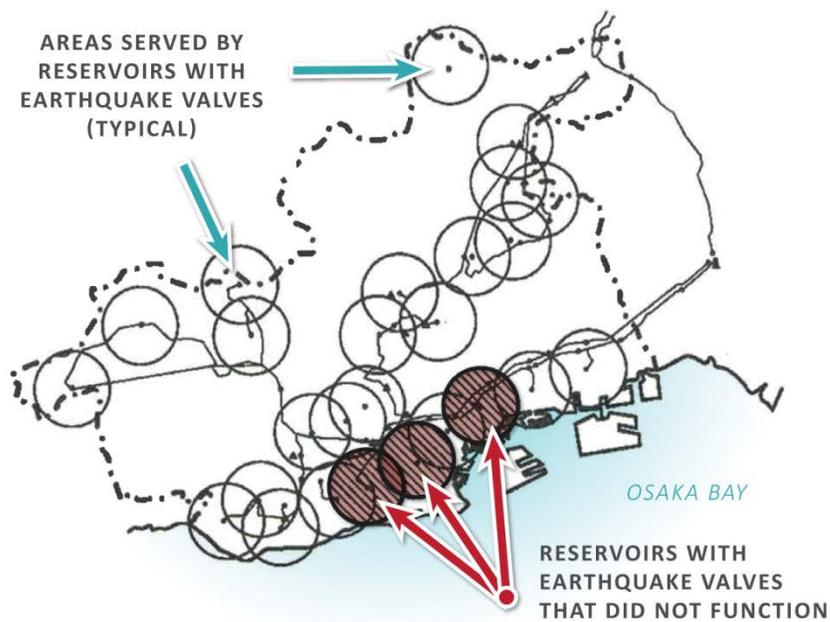
**Figure 2. Schematic View of Kobe Water Service Area Showing Reservoirs with Earthquake Valves and their Respective Service Area**
