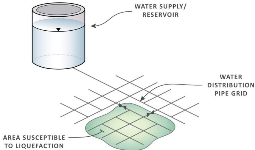
**Figure 3. Schematic of system similar to San Francisco’s dedicated fire protection system Earthquake Hazards**
