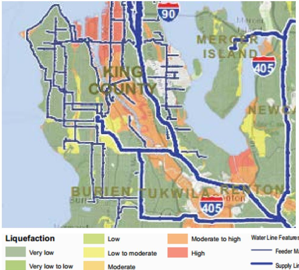
Figure 1. Example liquefaction map covering part of the Seattle water system
